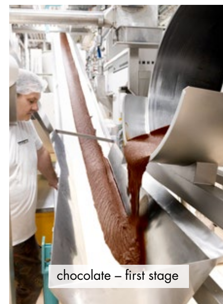
The final product after 20-30 hours inside of the conche
