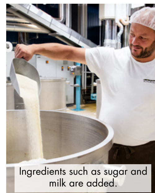
The bean-to-bar production space: the conche is in the foreground
